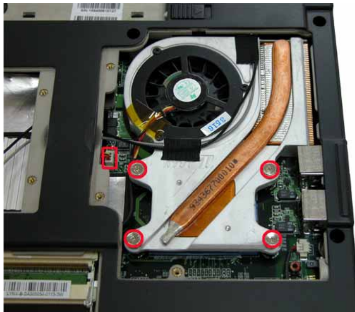
Fig. 11 Removing the screws retaining the heat plate
